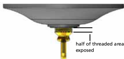
Drawing 2 Canopy Adjustment
