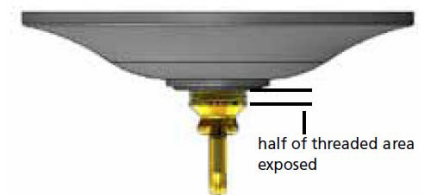
Drawing 2 – Canopy Adjustment
